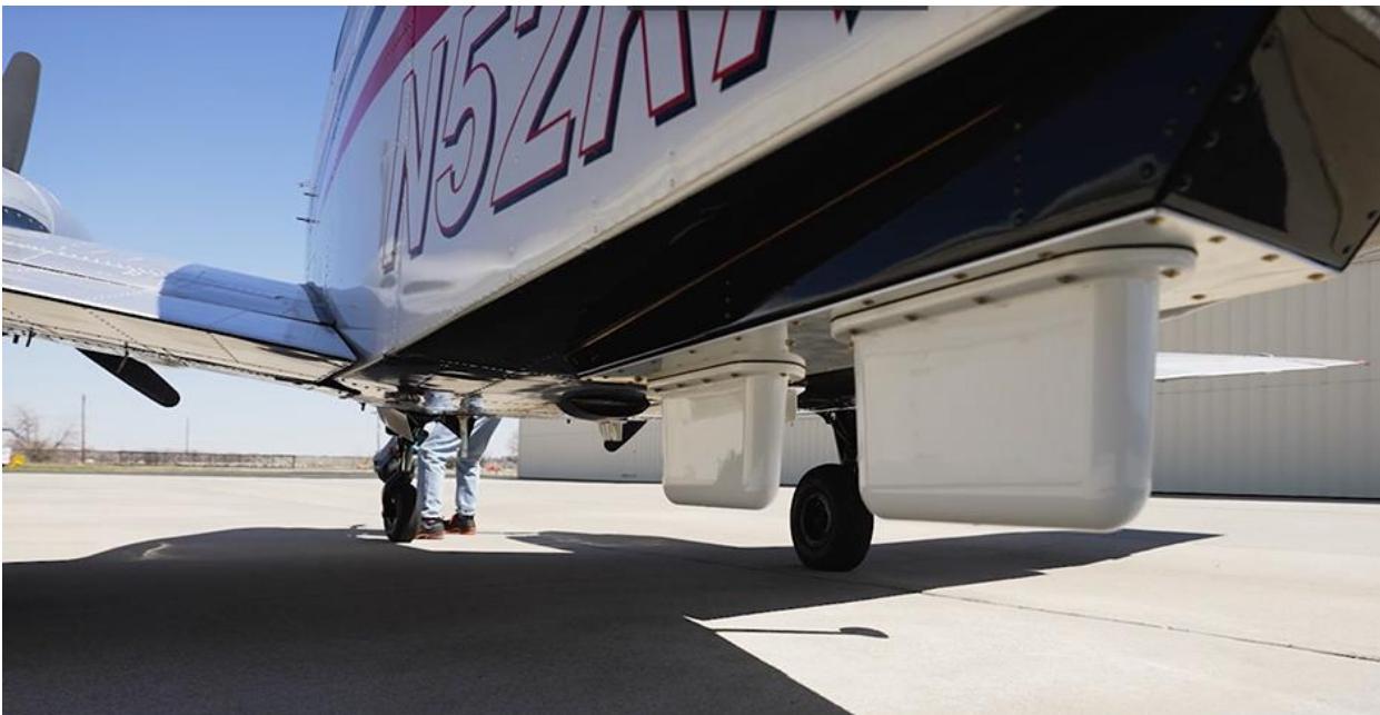
Image: Gogo 5G antenna mounted on the bottom of a private jet.
